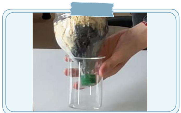
Picture 2. . Example of a “Do it Yourself” (DIY) purification system
